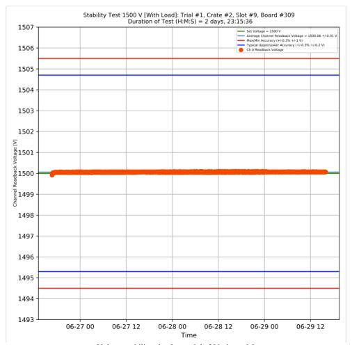
Voltage stability plot for module 309 channel 0
